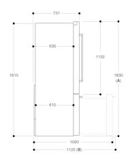
$\mbox{\bf A}\mbox{:}\mbox{ Front is adjustable from 1830 to 1847, with front levelling feet fully extended <math display="inline">\mbox{\bf B}\mbox{:}\mbox{ With handle}$
