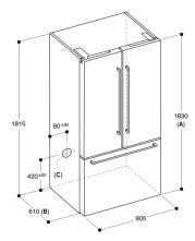
A: Front is adjustable from 1830 to 1847, with front levelling feet fully extended. B: Add 25 mm for fixed spacers on back
